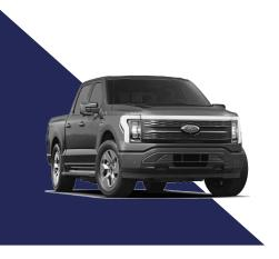
Despite that its average charging power between 10%-80% SoC of 145 kW is very similar to that of its pickup competitor Rivian and that their battery capacities are comparable, Ford F-150 Lightning's fast-charging capability is lower, especially until about 35% SoC. While the R1T maintains its charging power around 200 kW up to 35% SoC, the F-150 only charges up to 175 kW in that range.
