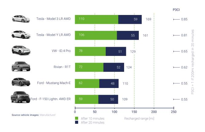
None of the EVs eligible for tax savings come close to the P3CI - US target value of 1.0. Tesla is ahead with the Model 3 Long Range AWD at 0.85 and the Model Y Long Range AWD at 0.81. Model 3 achieves the highest peak charging power (251 kW) in the com-
