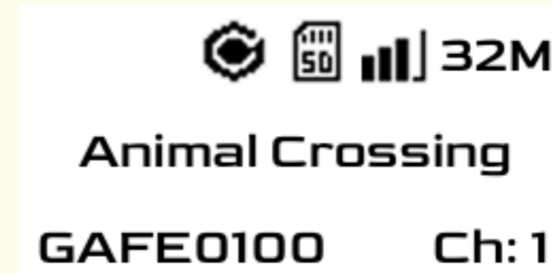
Fig. 1: The display during normal operation, showing the status icons at the top, loaded VMC name in the middle row and GameID and selected channel at the bottom row.
